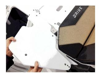
Fig. 48. How the rear sundeck should be installed.
