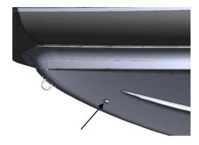
Fig. 6. Bow anchor drainage.
