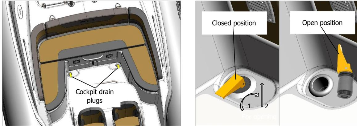
Fig. 3. Cockpit drainage.
