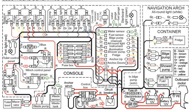
Fig. 62. Electrical schematic diagram.
