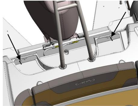
Fig. 33. Rear lifting eyes, 2 positions.
