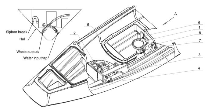
Fig. 40. Waste water system.
