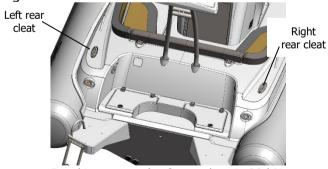
Breaking strength of rear cleat is 20 kN.
