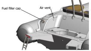
Access to the top part of the fuel tanks, as well to the connections and fuel sensor is provided through the hatch located on the deck and fixed by the screws. To get the possibility to unscrew and then open the hatch, helm and passenger double seat should be removed.
