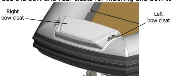
Breaking strength of bow cleat is 24 kN.
