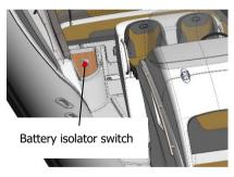
Fig. 27. Battery isolator switch.
