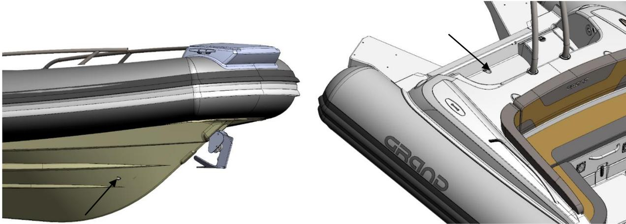
Fig. 6. Bow anchor and recess drainage.
