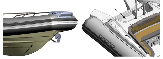
Fig. 6. Bow anchor and recess drainage.
