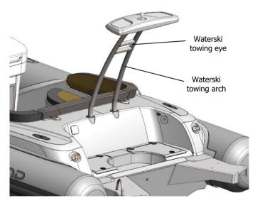
Fig. 46. Waterski towing arch.
