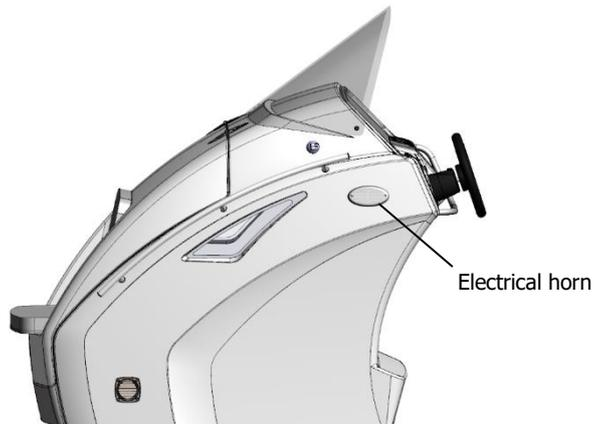
Before making a trip, check the horn is functioning by briefly switching it on/off.
