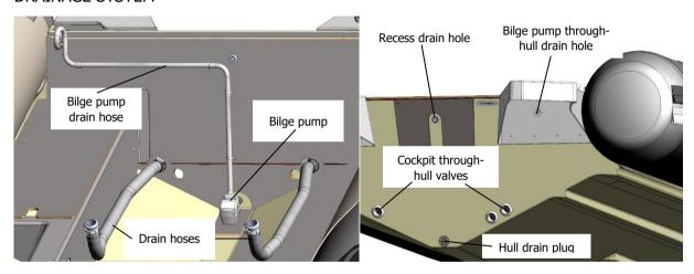
Fig. 2. The drainage system.
