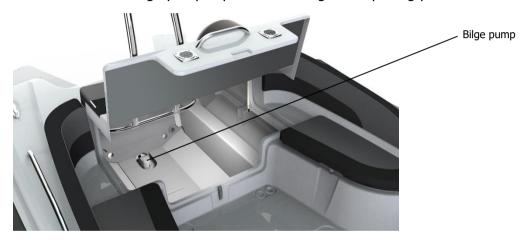
Fig. 5. Bilge pump and its location.
