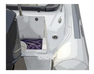
Fig. 42. Rear side rope hatches.
