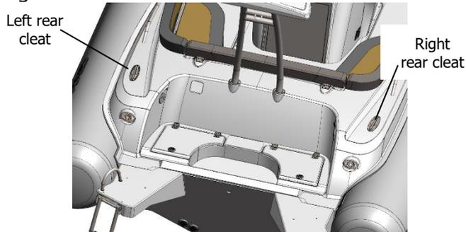
Breaking strength of rear cleat is 20 kN.
