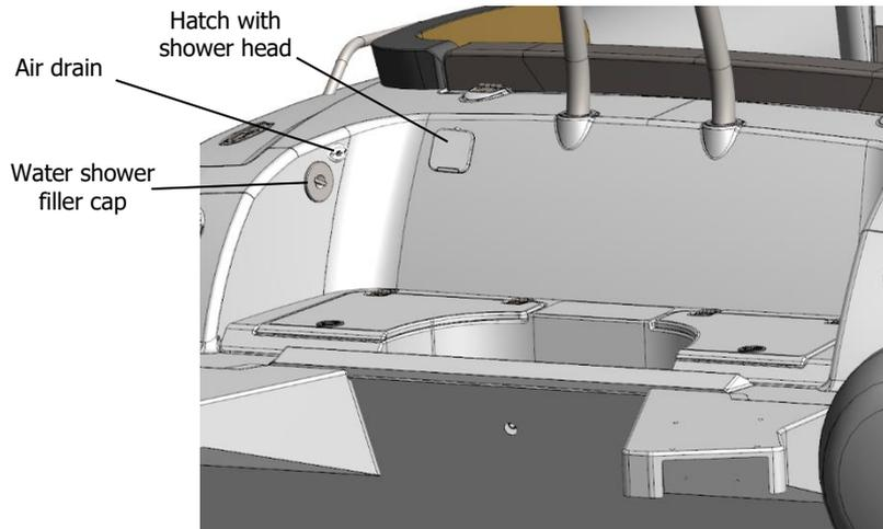
It is a good practice to rinse periodically the water supply system and fill up the water tank with freshwater after each use.
