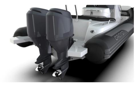
Fig. 53. Twin engine installation.
