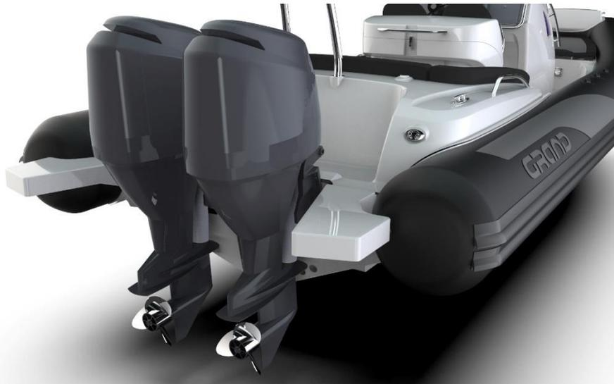
Fig. 53. Twin engine installation.
