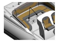
Fig. 9. Ventilation openings on the rear dry storage compartment.
