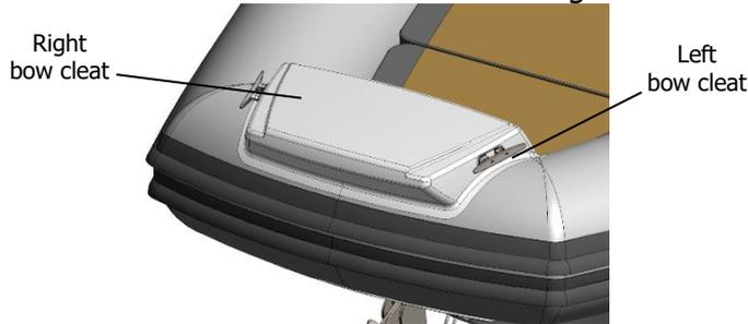
Breaking strength of bow cleat is 24 kN.
