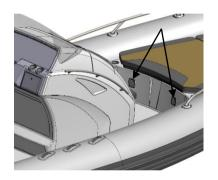
Fig.8. Ventilation openings on the bow compartment.
