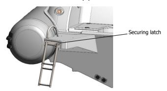
Fig. 49. Swimming platform with folding ladder.
