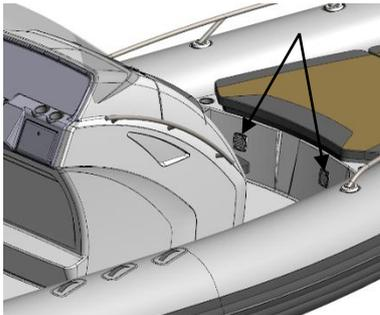
Fig. 8. Ventilation openings on the bow compartment.
