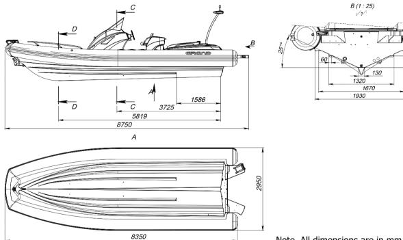
Fig. 64. Measurements for a correct trailer.
