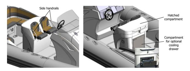
Fig. 35. Helm and passenger double seat with foldable seats.
