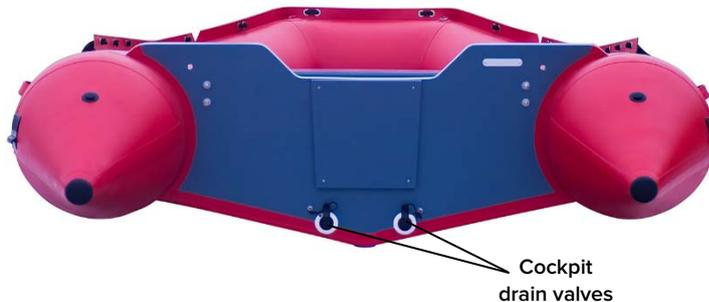
Fig. 1. Cockpit drain valves.
