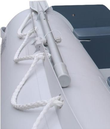
**Fig. 18.** Installation of oars.
